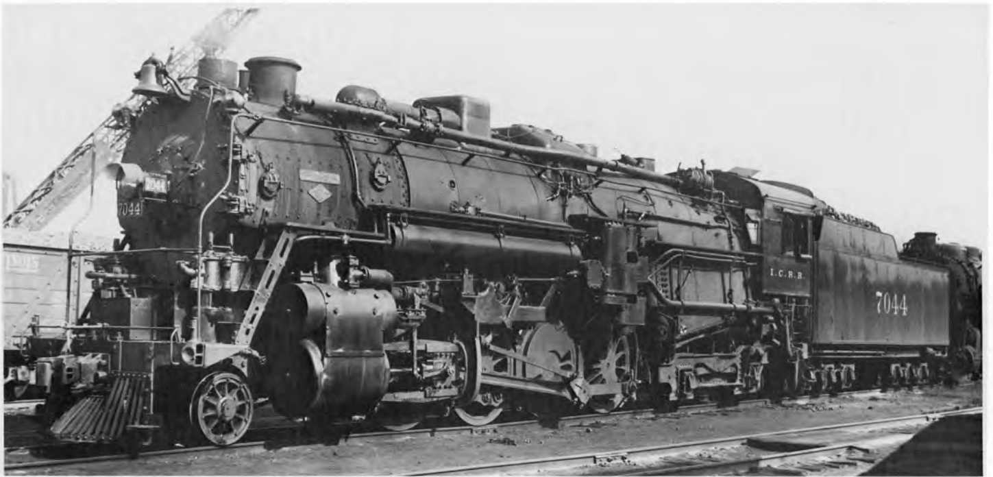
The 7044 at E. St. Louis, IL. showing the Worthington BL feedwater heater and a bell mounted high on the smokebox. Note also the riveted, shorter, open type pilot.
