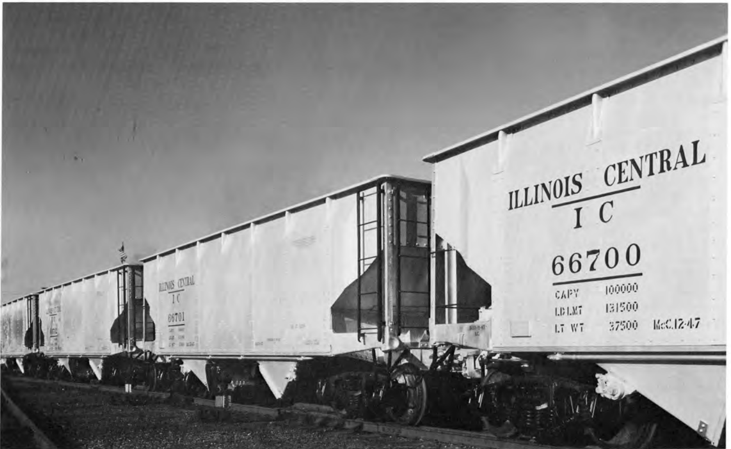
Here's a nice photo of IC's aluminum hopper car fleet. There were five cars total. Hedrich - Blessing photo, courtesy ICGRR.
