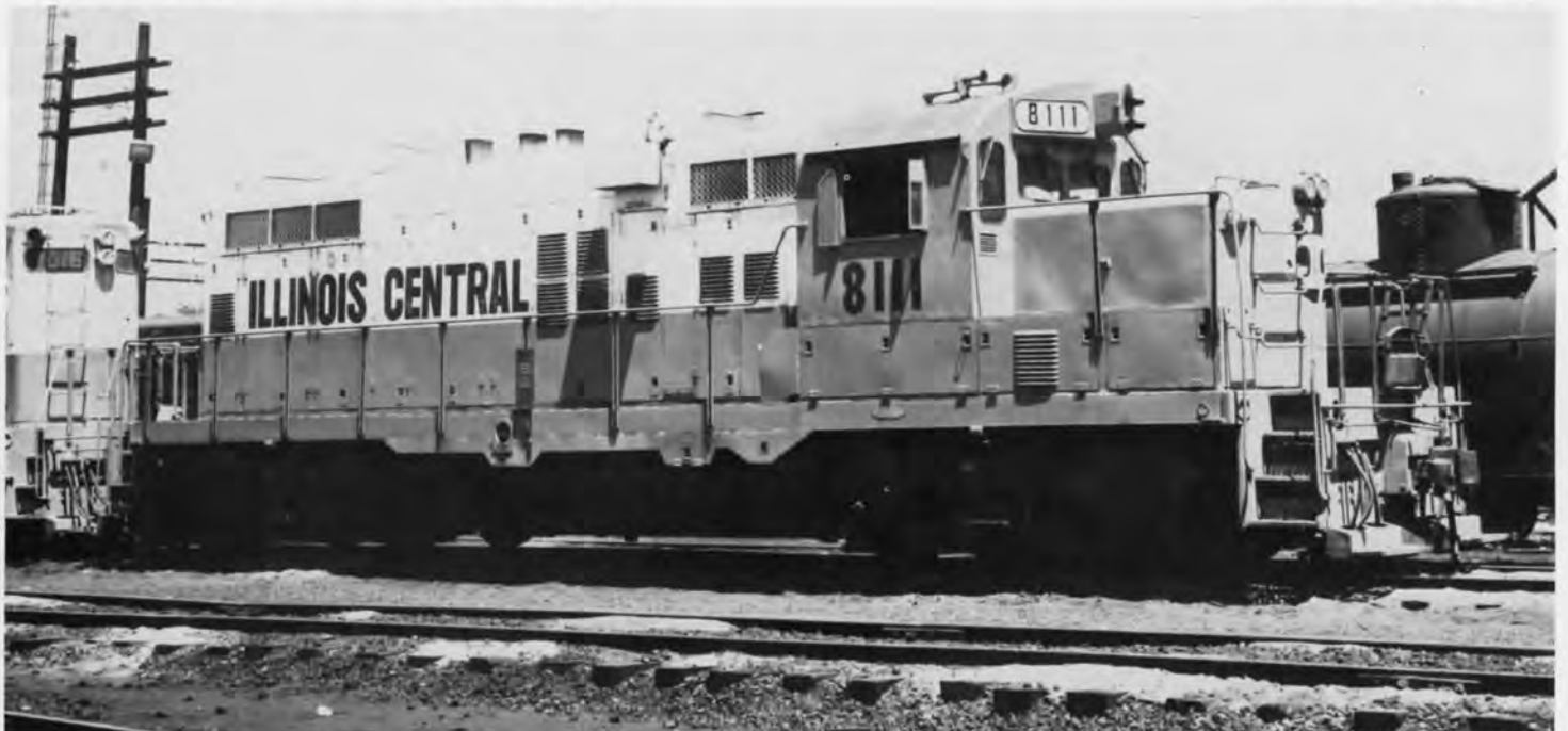
GP18 Paducah rebuild of a GP9 at Wamac IL in 1973.
