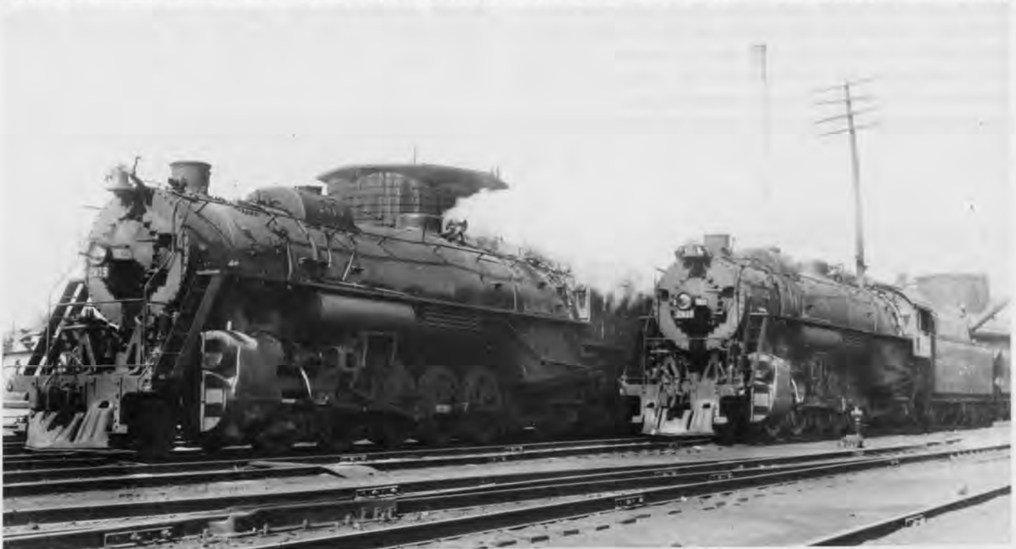
#2819 & #2810 at Waterloo Iowa, ready for their eastbound runs. Note the use of auxiliary tenders to eliminate water stops. Paul Slager photo.
