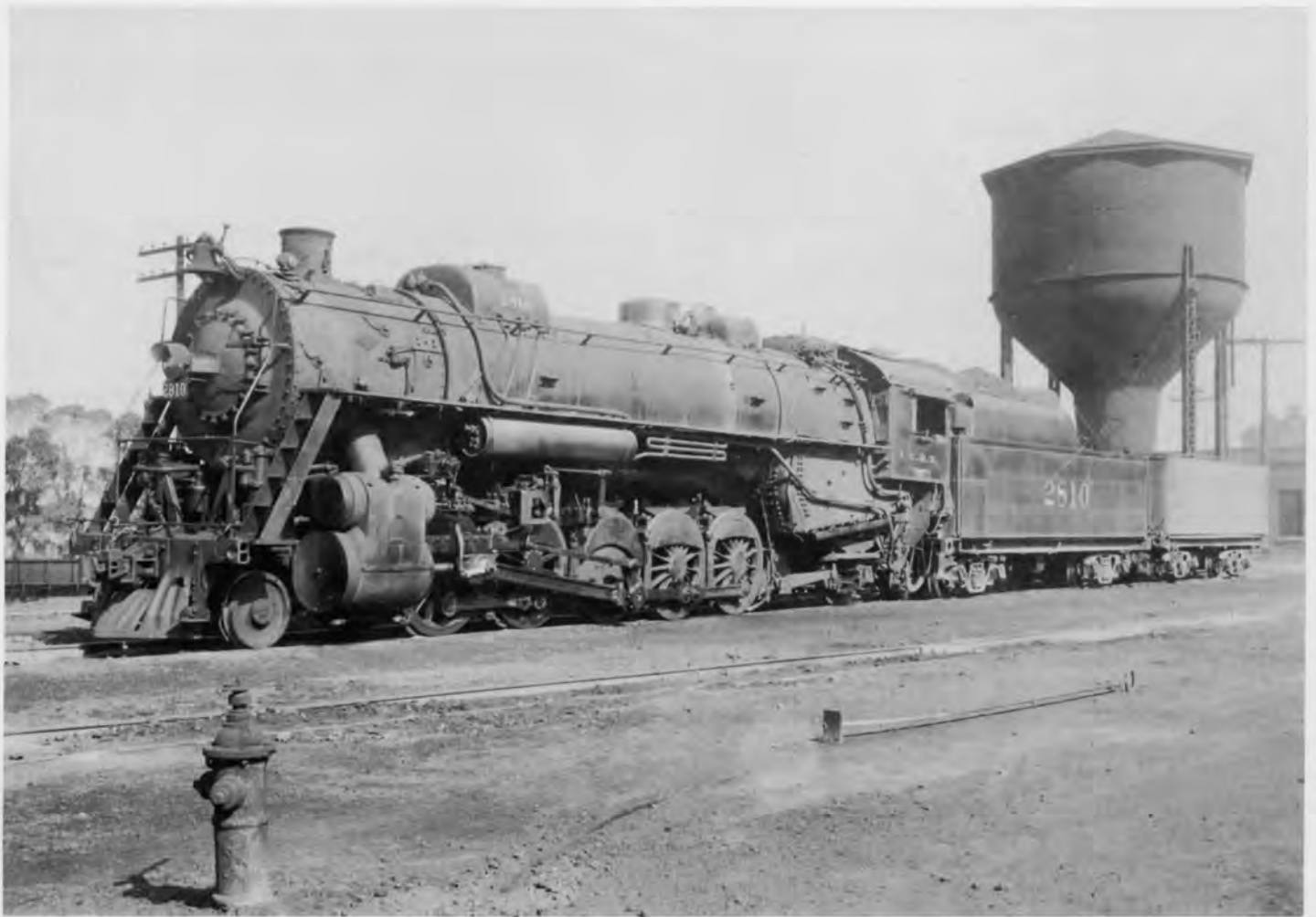
2-10-2 #2810 with an auxiliary tender sits ready for her next assignment. ICRR photo.
