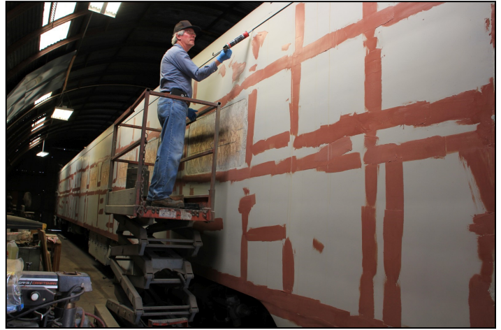
Bruce Backus seam seals diner 4110 after the first application of body filler during Spring Fling. Kent McClure photo
